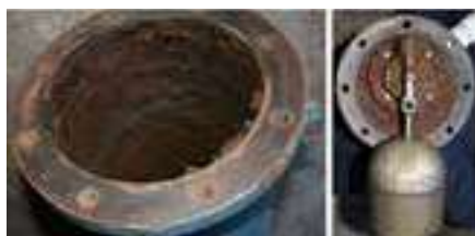
Figure 2 – Sludge build-up on uncoated internal valve casting.
