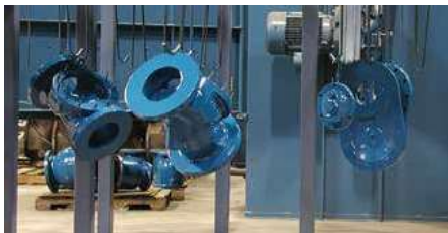
Figure 1 – Fusion bonded epoxy coating on valve castings.
